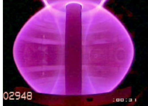
Fig.3. MAST: The additional tenuous plasma outside the main SOL disappears during ELM-free H-mode
